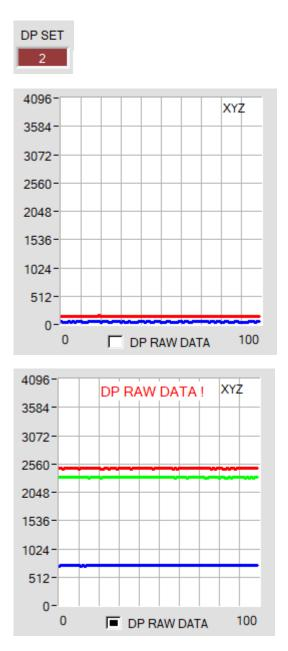
To understand with which **X**, **Y** and **Z** values the sensor works in parameter set 2, you can display this raw data in the display **XYZ** using the **DP RAW DATA** check box.
